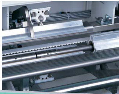
Open segment of the feed channel. View of the quick-change clip fastener, pusher, material in closed feed channel, material table
