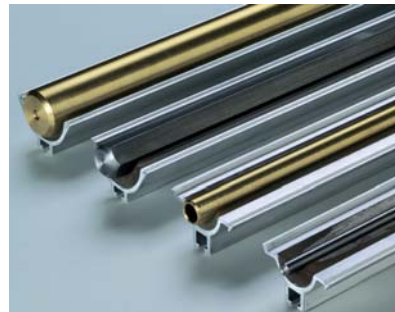
Feed channel segments (quick-change channels) for round and profiled bar stock. Lined with vibration-damping, highly wear-resistant synthetic material.
