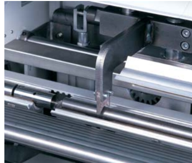
End piece ejection. The clamp releases the end piece from the clamping sleeve of the pusher
